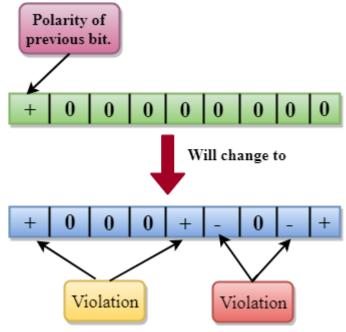
o If the polarity of previous 1 bit is negative, then the eight 0s will be encoded as zero, zero, zero, negative, positive, zero, positive, negative.
