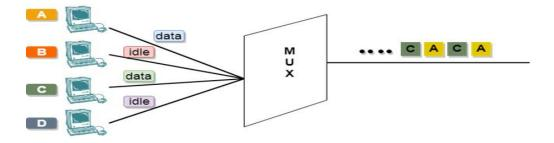
In the above diagram, there are 4 devices, but only two devices are sending the data, i.e., A and C. Therefore, the data of A and C are only transmitted through the transmission line.
