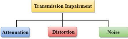
Attenuation: Attenuation means the loss of energy, i.e., the strength of the signal decreases with increasing the distance which causes the loss of energy.
