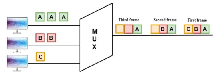
In the above figure, the Synchronous TDM technique is implemented. Each device is allocated with some time slot. The time slots are transmitted irrespective of whether the sender has data to send or not.
