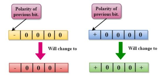
If the number of 1s bits is even, then the violation is made on the place of the first and fourth consecutive 0s. If the polarity of the previous bit is positive, then violations are negative, and if the polarity of the previous bit is negative, then violations are positive.
